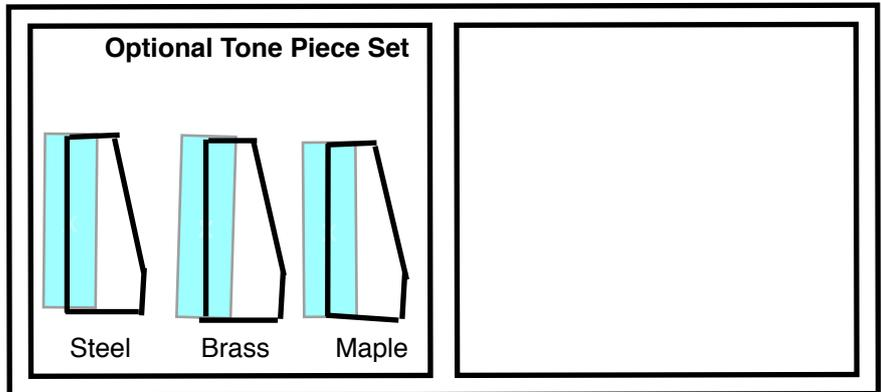
Optional tone pieces (above) can be used to replace the steel tone piece already on the tone amp **or added above it in a stack for greater volume**. Tape attached to all tone pieces should not be removed but reused as long as possible. To unstick any tone piece grasp it near the tape and lift it slowly. Store unused tone pieces in any space on the left.
